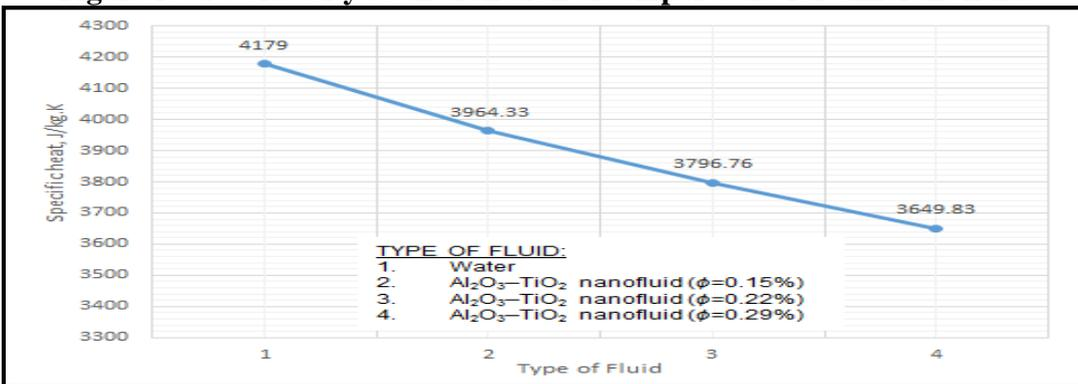
Figure No.8: Specific heat of various fluids
