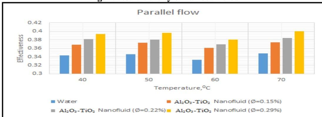
Figure No.10: Effectiveness of various fluids in parallel flow
