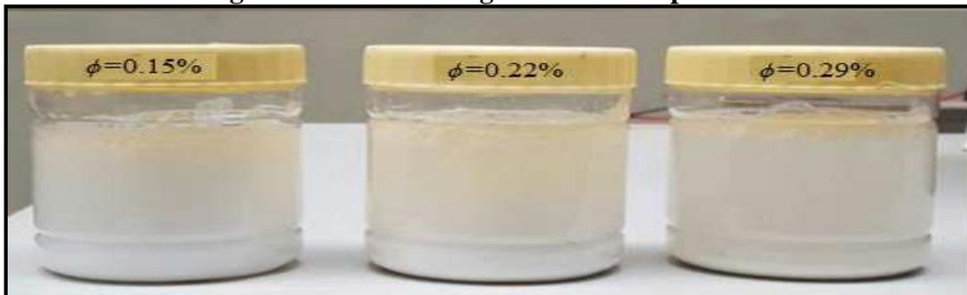
Figure No.3: Al<sub>2</sub>O<sub>3</sub>-TiO<sub>2</sub>nanofluid
