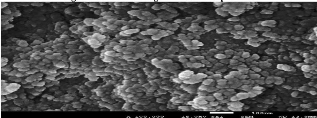
Figure No.2: SEM image of TiO<sub>2</sub> nanoparticles
