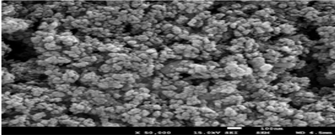
Figure No.1: SEM image of Al<sub>2</sub>O<sub>3</sub> nanoparticles
