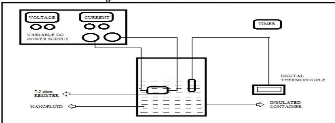
Figure No.4: Experimental setup of simple Calorimeter
