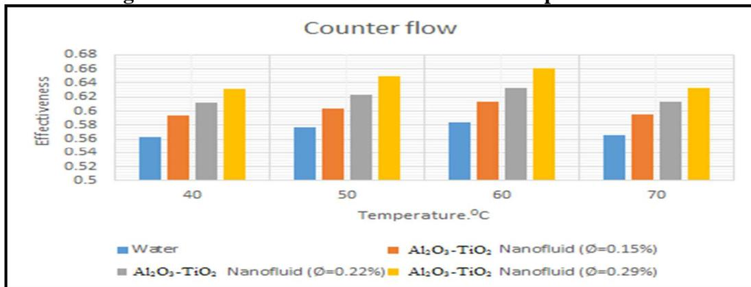
Figure No.11: Effectiveness of various fluids in counter flow
