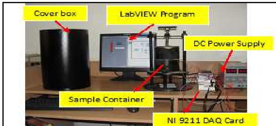
**Figure No.1: Experimental setup for transient heat plane source**
