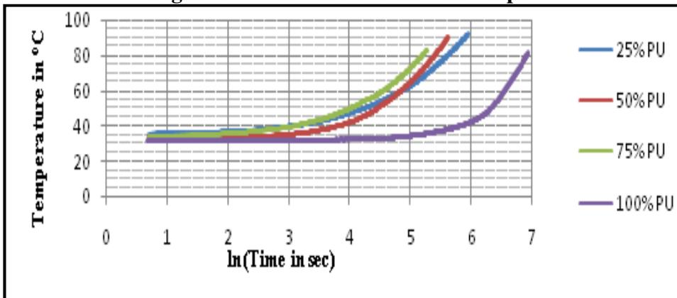
Figure No.4: Temperature in °C vsln (Time in Sec) for various concentration of Polyurethane foam
