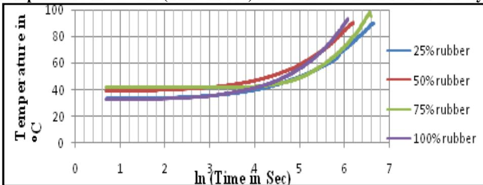
Figure No.5: Temperature in °C vsln (Time in Sec) for various concentration of Rubber foam
