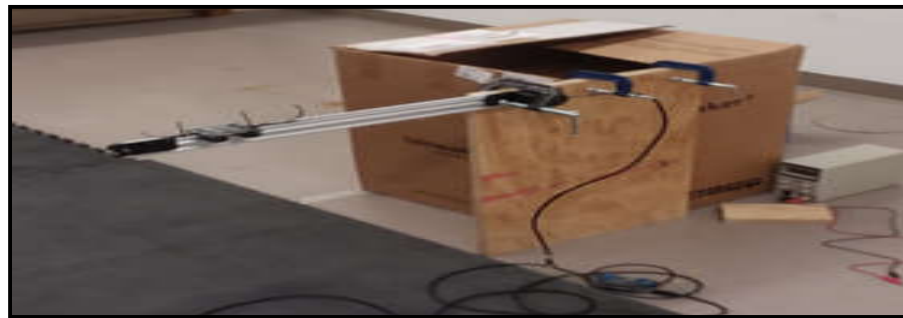
Figure No.5: Crazyflie 2.0 quadrotor used for test flights (top), linear actuator setup for collecting disturbance response data (bottom)
