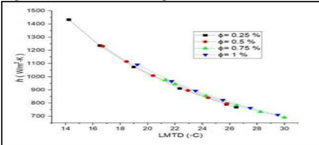
Figure No.4: Variation of Heat transfer coefficient with LMTD for different volume fraction of CuO nanofluid
