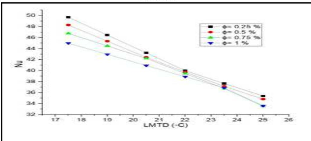
Figure No.5: Variation of Nusselt number with LMTD for different concentration of CuO nanofluid
