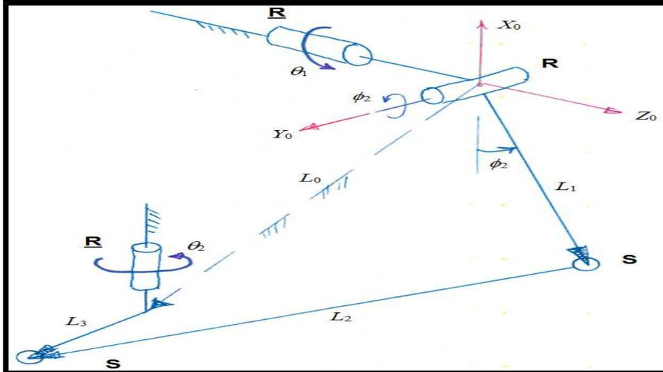
Figure No.4: RRSSR Kinematic Diagram for Left Hip
