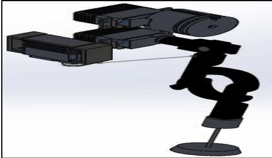
Figure No.2: RoboCat Left Leg CAD Model
